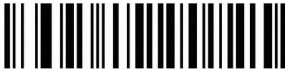
8 Bit, 2 stop Bit, No Parity
